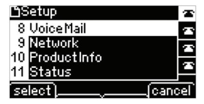
The IP address is displayed on the Network screen.
