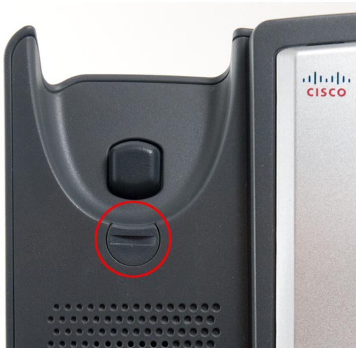
Figure 3 Handset Retention Tab (Default Position)
